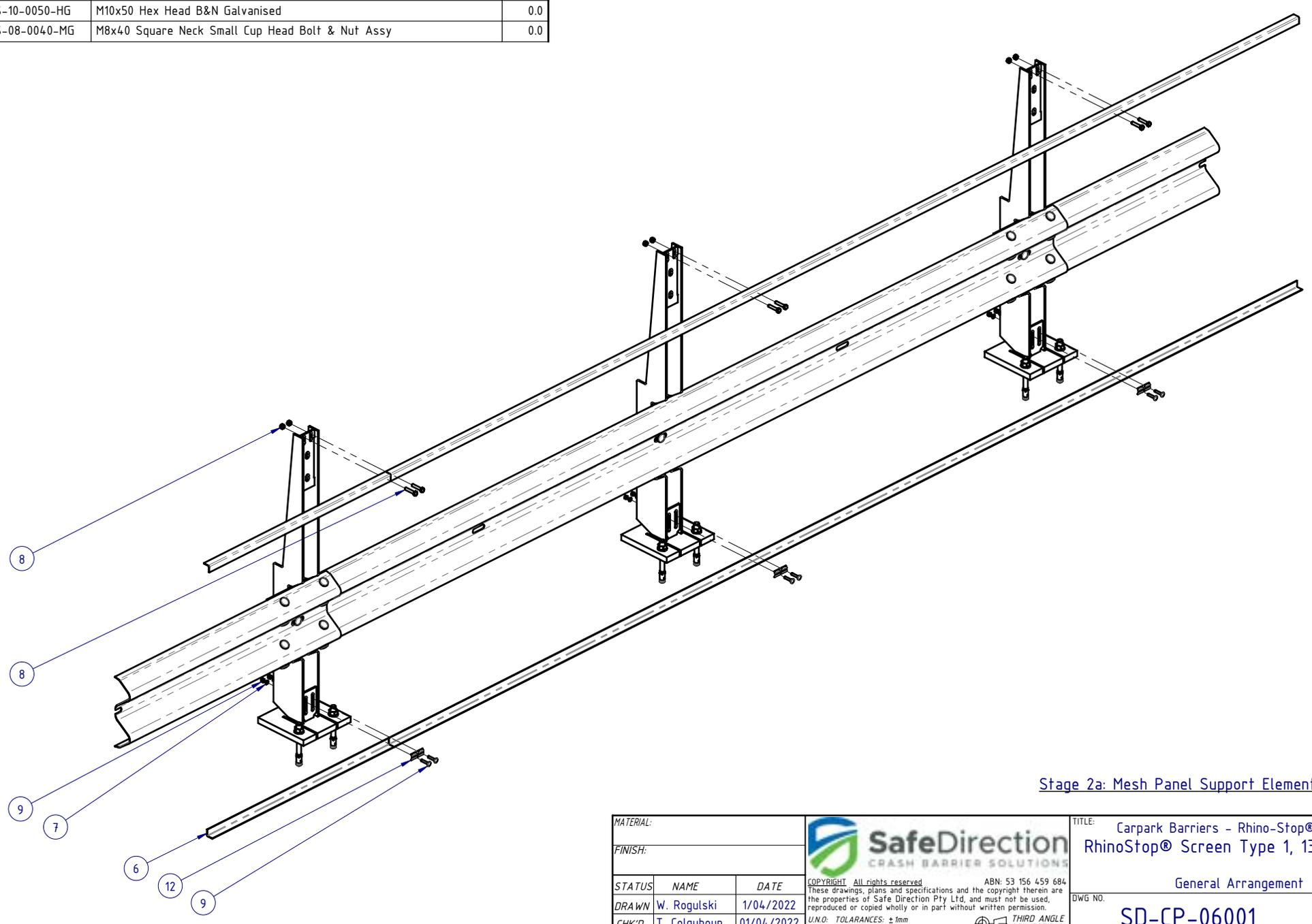
Stage 2a: Mesh Panel Support Elements Assembly
