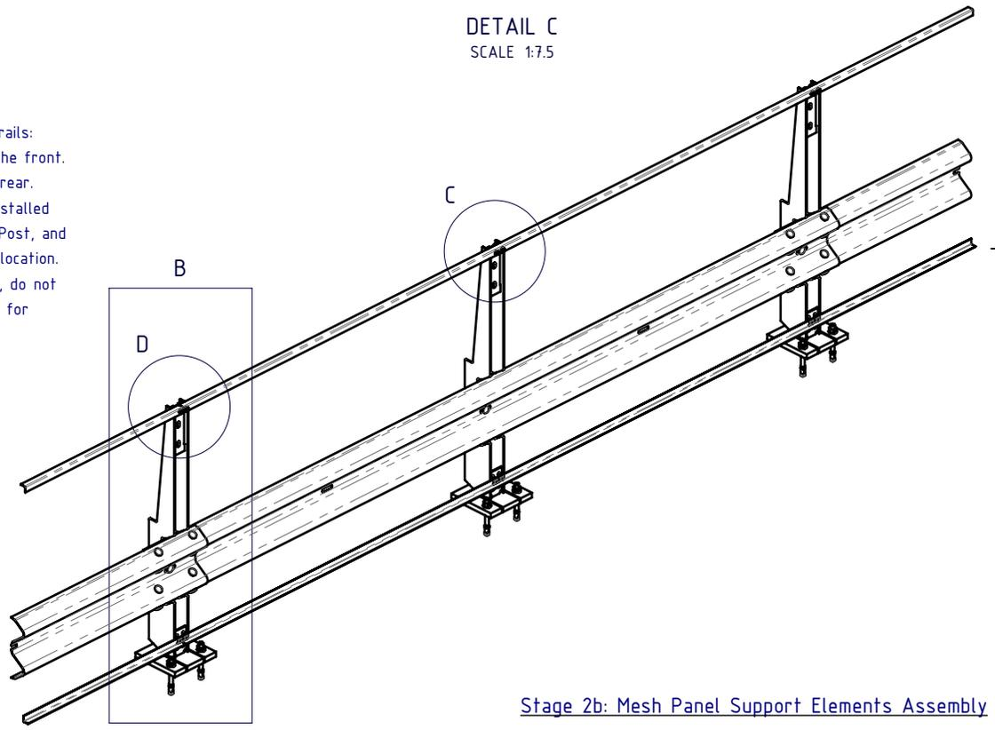
Stage 2b: Mesh Panel Support Elements Assembly
